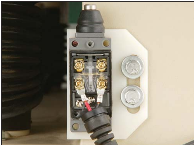
Figure 96. Lower table limit switch.
